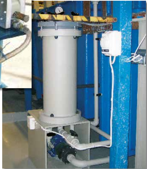
Filter FT and magdrive pump CTM used ▶ for circulation and filtering of surface treatment bath
