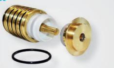
The TF series is equipped with a special, hybrid air valve comprising of a brass body and PET cylinder. The cylinder is made of a light material therefore it does not damage the air valve housing and the pump center body at high pressures.
